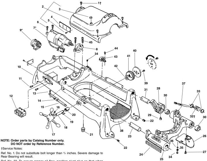
Ref. No. 32. To assure proper oil flow, position pivot plug so that when spout is in up position, oil flow hole is visible in carriage slot below spout.
